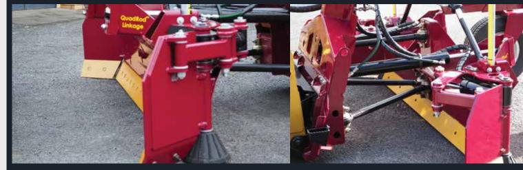
Cut, carry or windrow material forward or backward with double acting wings & rear blade
