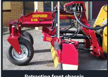
**Retracting front chassis** for reduced transport length
