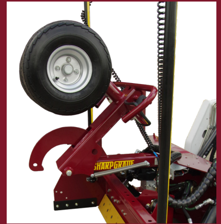
Retracting wheels for confined space / transport
