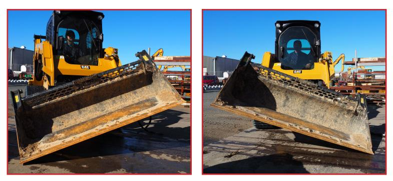
Fully controllable 22 degree left and right pitch
